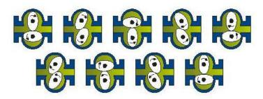
Each rotation of the oval wheels displaces four discrete volumes of liquid through the meter (between the oval wheel and measurement chamber).
