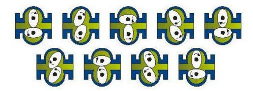
In each revolution, the oval wheels displace a discrete volume of liquid (that is defined by the space between the oval wheel and measuring chamber) through the chamber.
