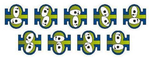
In each revolution, the oval wheels displace a discrete volume of liquid (defined by the space between the oval wheel and measuring chamber) through the chamber.
