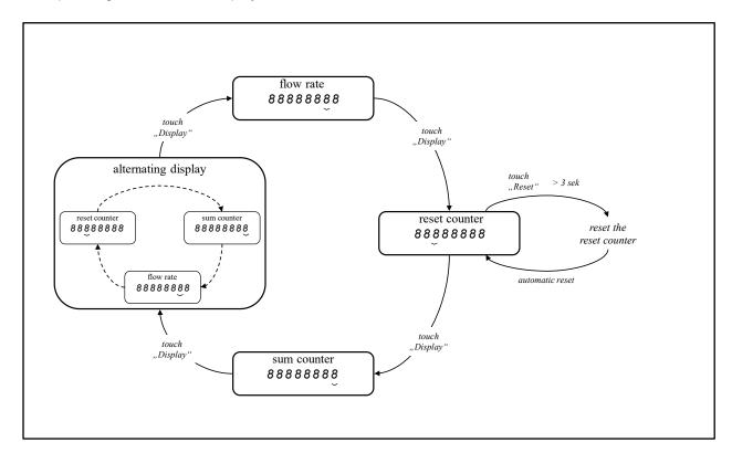
In the alternating display mode all three indications are activated sequentially at preset time intervals. The resetting of the reset counter can only be effected while this specific value is being displayed. The contact must be actuated for at least three seconds. For better legibility the display circuit board may be rotated mechanically by 90° or 180° (see also appendix B3).
