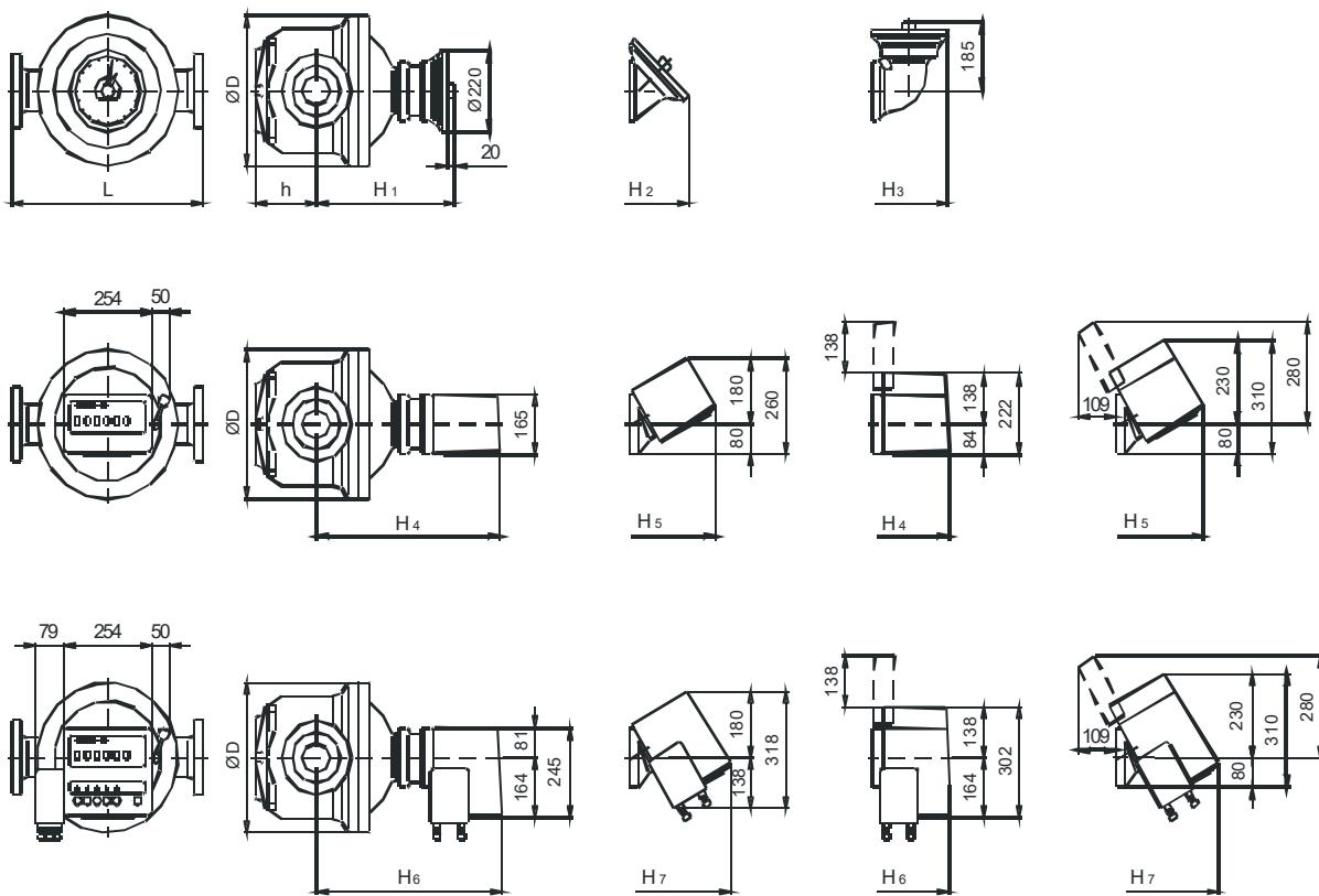
For counters with remote control, pulse pick-up AG 19/20/45 or extension dimensions H1 to H7 are:
