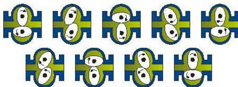
Each revolution of the oval wheels displaces four discrete volumes of fluid (defined by the space between oval wheel and measuring chamber) through the counter. For measuring purposes the rotation of the oval wheel is transmitted from the pressure chamber to the outside via an electromagnetic sensor according to the Wiegand principle and processed to be available as standardized electrical signal or counter display.
