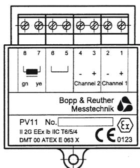
At the Terminals 8 and 7 the Sensor is connected internally.
