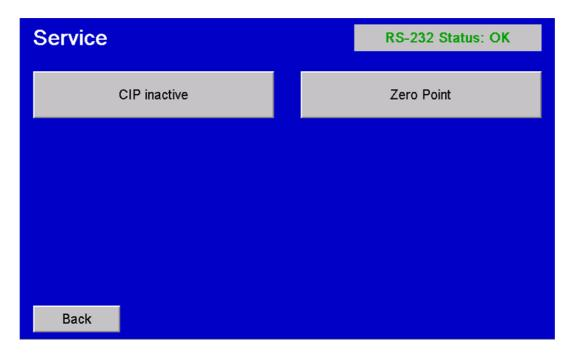
With the button "CIP" all valves will be opened after a confirmation message. The valves will open as long the "CIP"-button will be pressed again.
