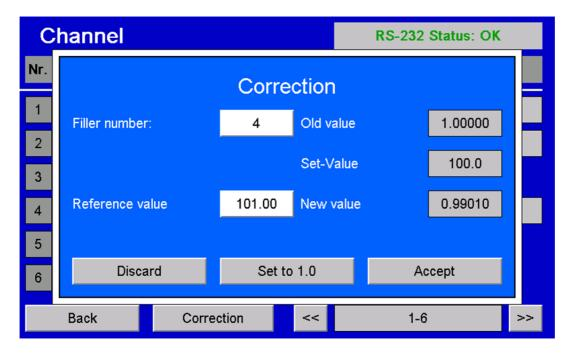
Shown below is a reference value of 101,00 g for the channel 4. After the input the button "NEW" appears on the right side. Press this button and the correction value will be calculated and the reference value get erased again.
