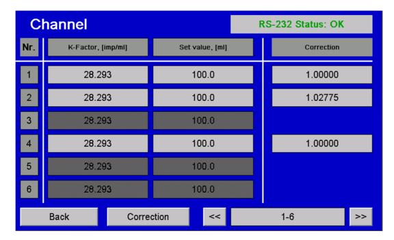
By entering the reference value, it is possible to assign a correction factor to each channel separately.
