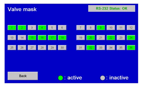
E.g.: Here on the picture 36 channels are given, whereby only 1-2, 4, 9,15-18, 20, 22, 24, 32, and 36 are active.
