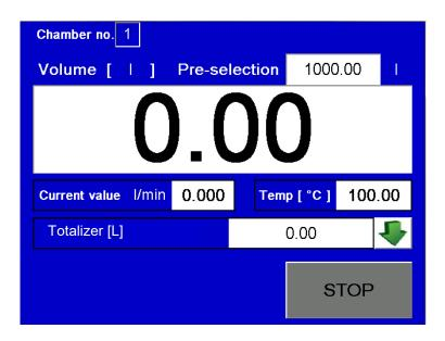
The large display (volume at operating temperature) has been selected in advance and the small window can display the quantity at 15° C or the volume at the operating temperature or the calculated mass.
