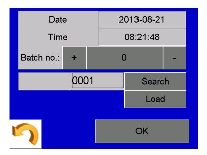
If a loading is retrieved from the batch memory, all the relevant data is displayed on the screen, e.g. date, time, quantity at loading temperature, standardized volume, mass, determined temperature via loading, etc.
