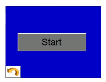
The screen shown above is the start-up screen and appears at "New start-up" as well as after "Power failure" and also after filling, provided this has been completed correctly.
