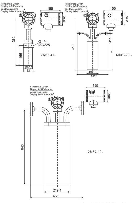
1) overall length DIMF 1.3 in flange design 200 mm 2) overall length DIMF 2.0 in flange design 250 mm
