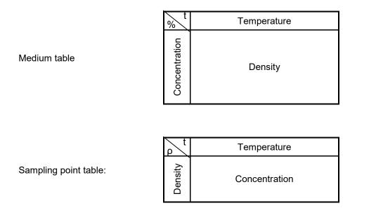
The table is transferred to the density meter during production.
