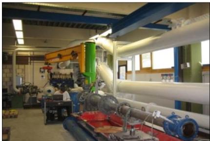
For calibration of oval wheel and turbine meters, vortex meters and vortex meter run, mass flow meters, orifices, nozzles, venturi nozzles, complete differential pressure meter runs up to DN400
