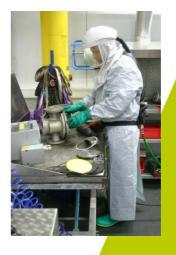
In our diagnostic area, measuring instruments and fittings are decontaminated in accordance with VCI guidelines. We are audited by one of the largest chemical companies in the world and approved for the repair of contaminated measuring instruments.
